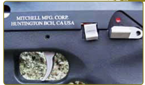
The toggle safety and bolt release button are handy, but not "thumb handy."
